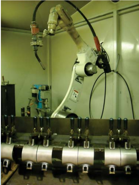
All PipeKlamps feature high quality robotic welded lugs for added strength and less deformation.
